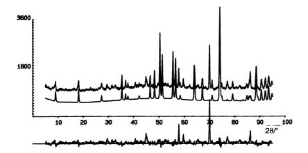
Fig. 1. Profile fit of neutron powder diffraction data. Upper curve observed and lower curve calculated profile. Differences are given in the lower part of the figure. The two sharp reflections at  $2\theta$ =59 and 70° are the (111) and (200) reflection from Al. The remaining peaks in the difference plot are from unidentified impurities, and none of these reflections can be ascribed to  $Tl_2Ba_2CuO_{6+y}$  or  $Tl_2Ba_2Ca_2Cu_3O_{10+y}$ .
