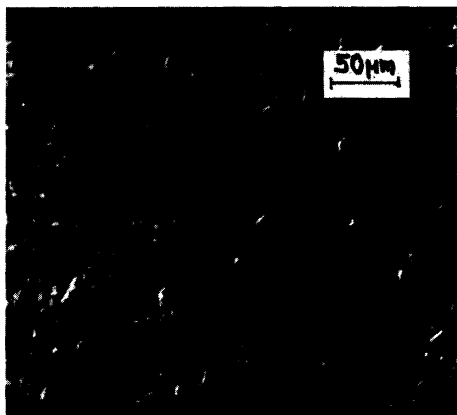
Fig. 1. Surface of the Al layer deposited in an electrolyte containing 80% \text{AlCl}_3 + 10% \text{NaCl} + 10% \text{KCl} at 180 °C at a current density of 3 \text{A dm}^{-2} .
