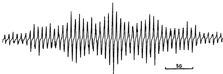
Fig. 2. The simulated EPR spectrum of the anion of Fig. 1 (based on Table 1 and the line width of 0.08 G).
