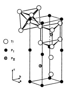
Fig. 1. The crystal structure of TiP.
