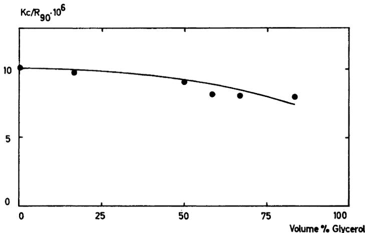
Fig. 4. Same as Fig. 3 but for bovine serum albumin in water (actually 0.1 M acetate buffer, pH 4.4)-glycerol mixtures.
