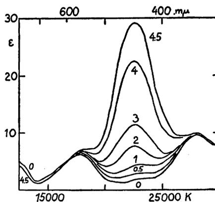
Fig. 1. The absorption spectra of 0.1 M Ni trien( $\text{NO}_3$ )<sub>2</sub> in water and aqueous solutions of sodium perchlorate. The numbers on the curves indicate the molarity of  $\text{NaClO}_4$ . The spectra were measured at 19°C on a Cary spectrophotometer.
