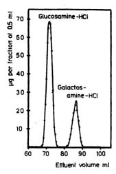
Fig. 1. Separation of 500  $\mu g$  glucosamine-HCl and 225  $\mu g$  galactosamine-HCl. Column 0.7  $\times$  39.0 cm.
